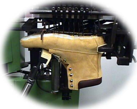
ASF-A Curing Station closeup Tru-Fit® Shank formed, hardened and bonded to lasted shoe bottom
